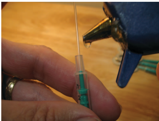
Figure 3. Hot Glue Added to Capillary Tube Base
