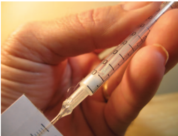
Figure 4. Cotton Inserted into Microrespirometer Barrel
