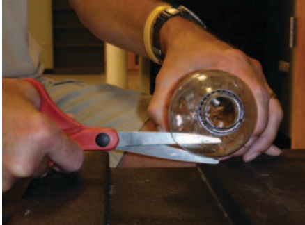
Figure 1. Notice that the scissors are cutting along the bottom of the bottle curve. This provides better control.
